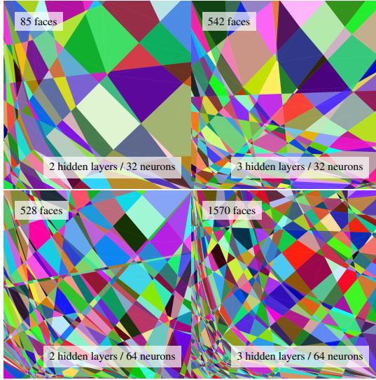
Figure 6: The number of faces of subdivisions of the bilinear function for different MLP configurations: the number of hidden layers and the number of neurons in each hidden layer.
